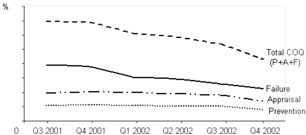
Figure 2: CoQ in manufacturing operations for Company A shown on a relative cost scale.
